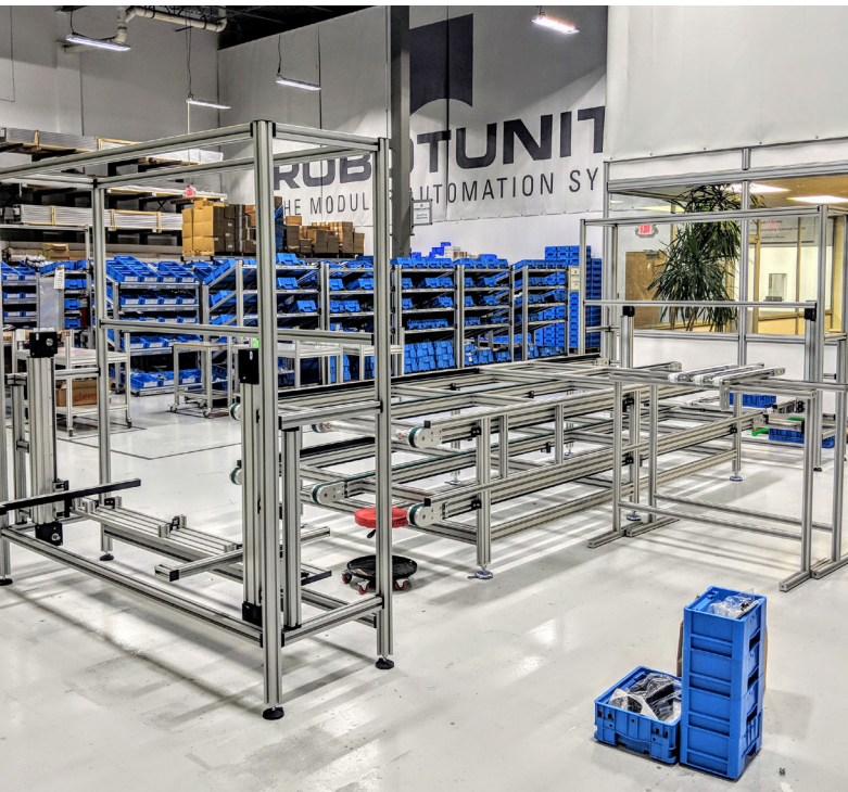
A custom configuration of Timing Belt Conveyors and Lift Station.
