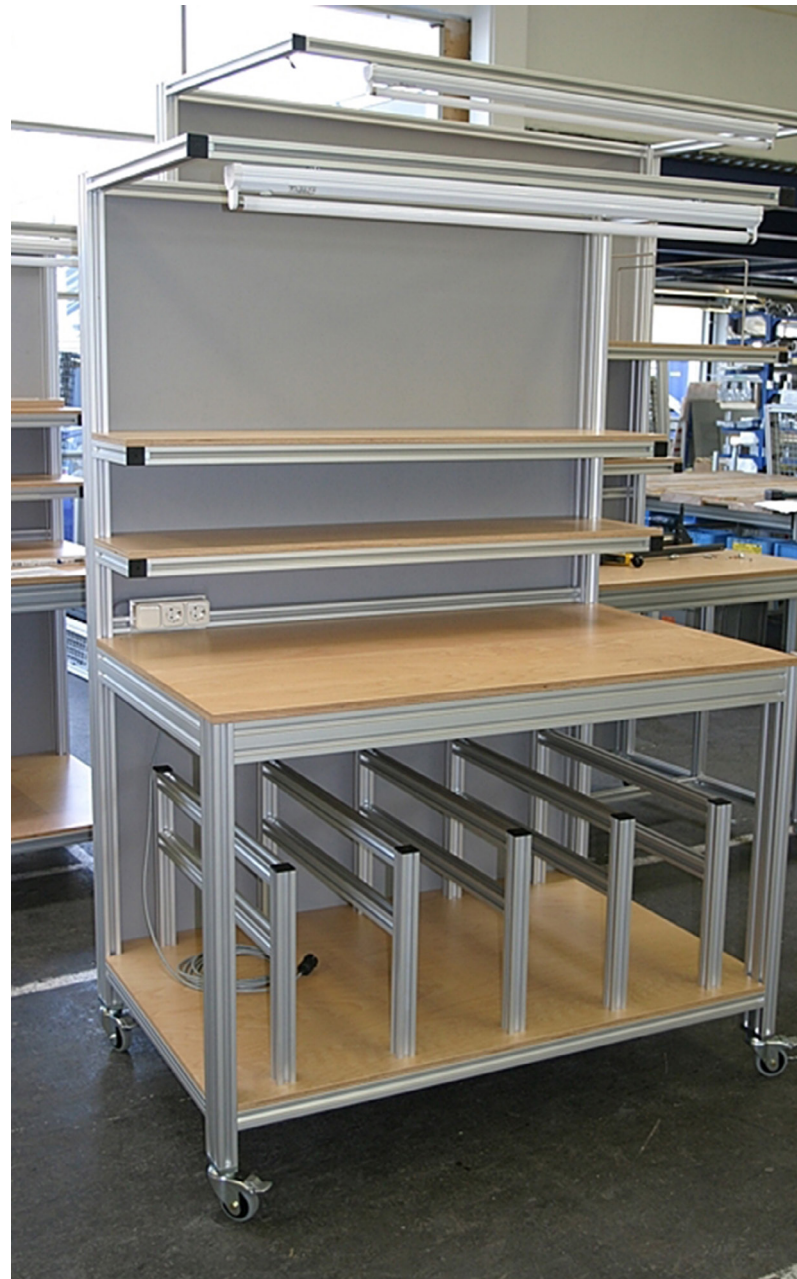
Robotunits' Extrusion and Fastening Technology, based on a common 14-millimeter T-slot, makes it easy to create a custom workstation — such as this rolling unit with lightbar — for your lean manufacturing operation.
