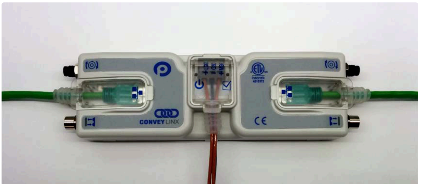
Ai2 Module with Left & Right Ethernet Cable with Covers attached
