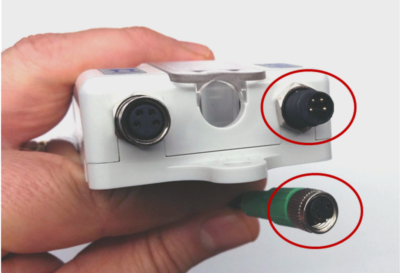
M8 4 Pin Male Motor Port with Senergy Ai Motor Female Connector
