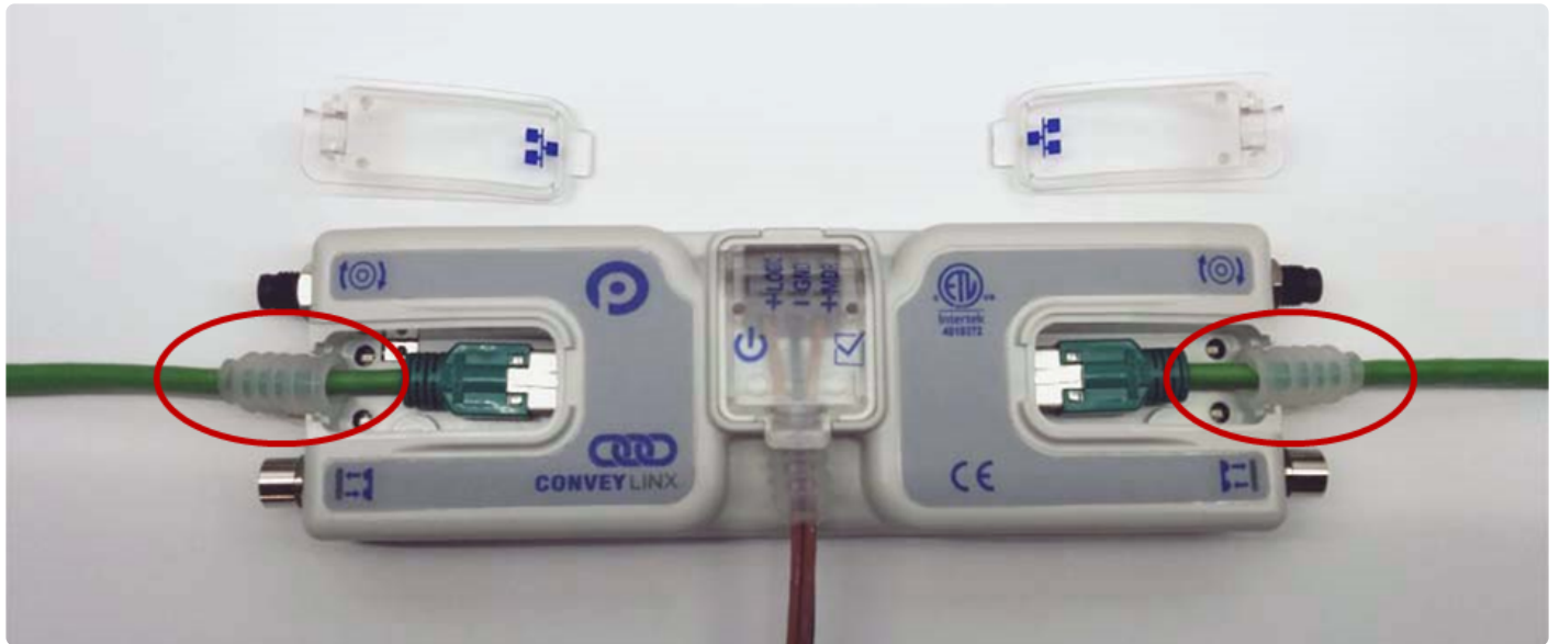
Ai2 Module with Left & Right Ethernet Cable (Covers removed)
