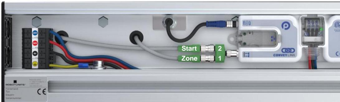
The zone and start sensor of the first zone must both be connected with a 3-pin cable. A Y-distributor is attached to the controller, to which both 3-pin cables are then connected.
