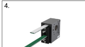
4. Pull out and replace belt
