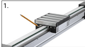
1. Loosen belt tensioner unit
