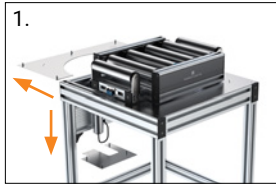
Remove the motor-side protection guard
