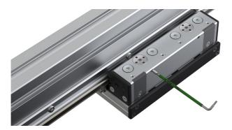
4.3.2. Use an Allen key to align the eccentric roller with the guide rail without applying force
