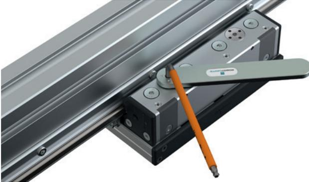
4.3.5. Fix the set screw to secure the excenter nut
