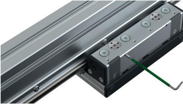
4.3.2. Use the Allen key to let the eccentric roller line up on the guide rail without expenditure of force.
