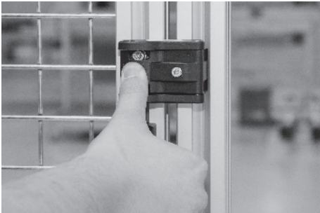
Secure: Push latch to open door.
