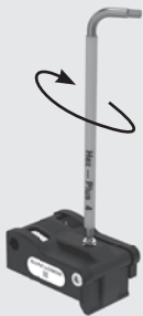
Adjustable pre-tension for optimal retention force. Set screw must always protrude by at least 2 mm.
