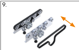
Remove the side panel and replace the belt
