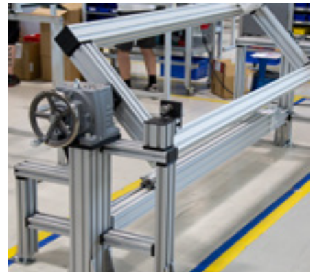
Workbench - adjustable via hand crank
