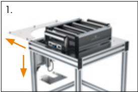
Remove the motor-side protection guard
