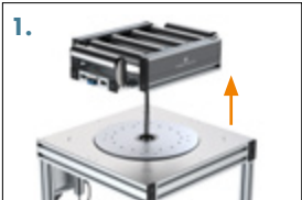
Remove powered roller conveyor incl. wiring
