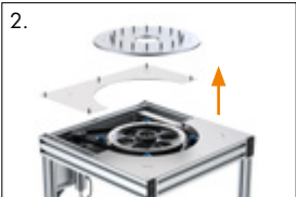
Remove the protection guard and driver plate
