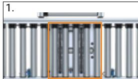
Remove rollers in the area of the Transfer Unit 90°
