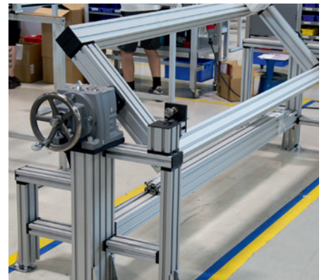
Workbench - adjustable via hand crank
