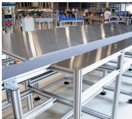
Workbench with integrated belt conveyor
