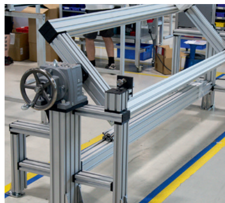
Workbench - pivotable via hand crank
