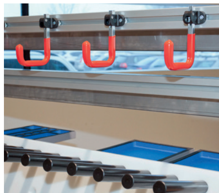
Expansion possible via attachments using the 14 mm slot
