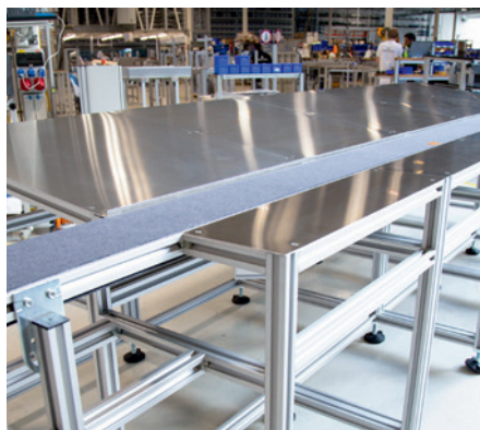
Workbench with integrated belt conveyor
